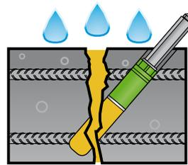
If moisture penetrates through the cracks, e.g. in basements, those cracks are likely to cause a limitation of the functionality of the building. This often happens with large concrete construction members, like tunnels or parking decks, especially if there are not enough expansion joints. If there are active leakages, those have to be
